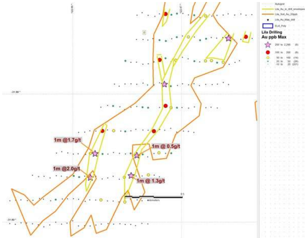
Lila Drill intercepts, with two mineralised horizons, and envelope of Au in soil >20ppb.
